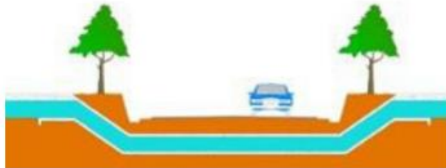
Gambar III.14 Bangunan Siphon Drainase
