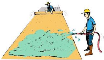
Gambar 3.22 Curing Beton
